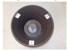
I made three brackets to attach the disk and mounted it on the pot. I then added an aluminum angle to the antenna base and fastened it to the disks.
